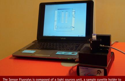
The Sensor Fluoralys is composed of a light sources unit, a sample cuvette holder to be filled with the crushed or liquid food and a spectrometer to analyse the emitted signal. The software allows the translation of the signal into NFC concentration
